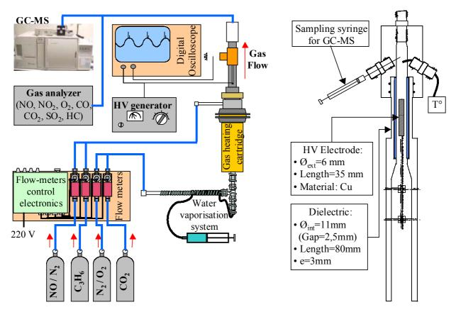
*Fig. 1. Experimental set-up of the wire-cylinder reactor, gas feeding system and analysis apparatus*
