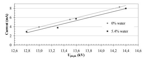
**Fig. 4.** Current vs. voltage curve obtained for the treatment of the  $O_2$  (10%),  $CO_2$  (10%),  $H_2O$  (0 or 5.4%),  $C_3H_6$  (1000ppmv), NO (1000ppmv) and  $N_2$  (balance) gas mixture (T=100 to 180°C depending on discharge power, flow=12.9 slpm)
