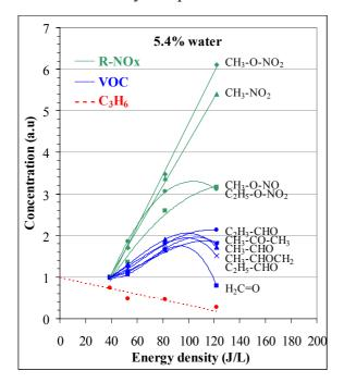
Fig. 7.1 and Fig. 7.2 indicates the relative concentration vs. energy density of the different analyzed species.
