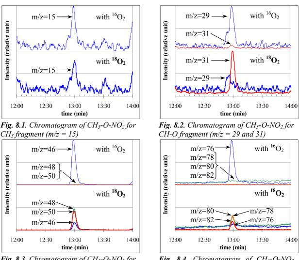
Fig. 8.3. Chromatogram of  $CH_3$ -O-NO<sub>2</sub> for NO<sub>2</sub> fragment (m/z = 46, 48 and 50)
