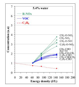
**Fig.** 7.2. Quantitative variation of  $C_3H_6$ and by-products depending on energy density for an  $O_2$  (10%),  $CO_2$  (10%),  $C_3H_6$ (1000ppmv), NO (1000ppmv) and  $N_2$ (balance) dry gas mixture (T=100 to 180°C depending on discharge power, flow=12.9 slpm)
