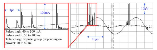
**Fig. 3.** Oscillogram obtained for the treatment of the  $O_2$  (10%),  $CO_2$  (10%),  $H_2O$  (5.4%),  $C_3H_6$  (1000ppmv), NO (1000ppmv) and  $N_2$  (balance) gas mixture ( $U_{pkpk}=14.5kV$ , frequency=44kHz, T=180°C, flow=12.9 slpm)
