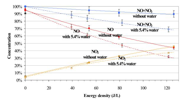
**Fig. 5.**  $NO_x$  concentration vs. energy density of the dry or hydrated  $O_2$  (10%),  $CO_2$  (10%),  $H_2O$  (0 or 5.4%),  $C_3H_6$  (1000ppmv), NO (1000ppmv) and  $N_2$  (balance) gas mixture (T=100 to 180°C depending on discharge power, flow=12.9 slpm)
